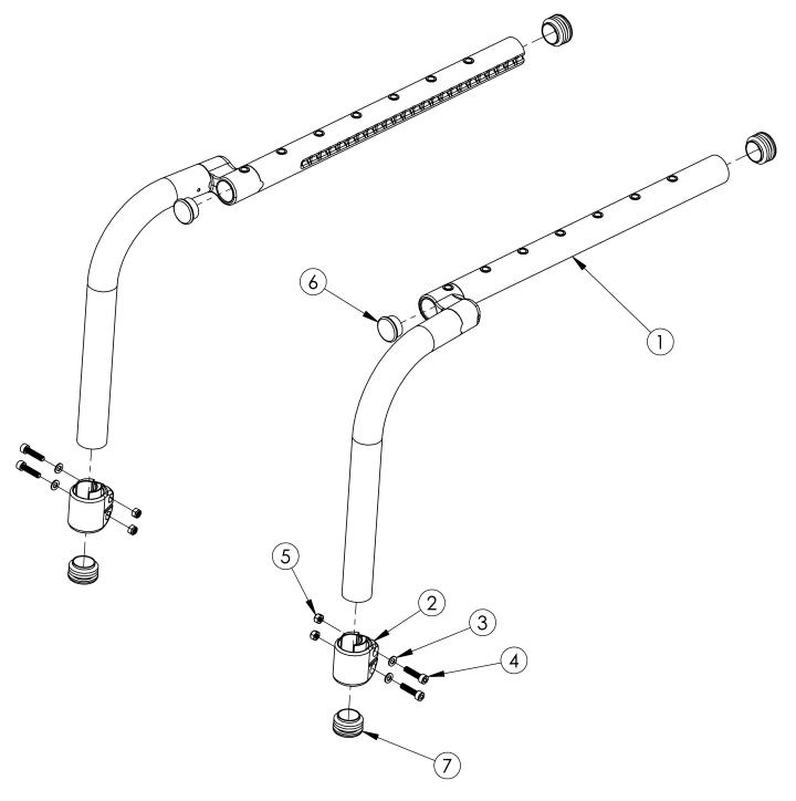
This Clik Offset Side Frame is discontinued and was used on serial numbers prior to CLK005270. Item numbers 2-5 are only needed when footrest is not high mounted.
