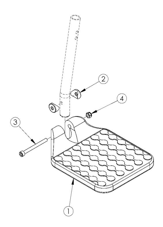
Sizes for footplates are based on seat width. If changing footplate style, new extension tubes may be needed. Only compatible with extension tube hangers.
