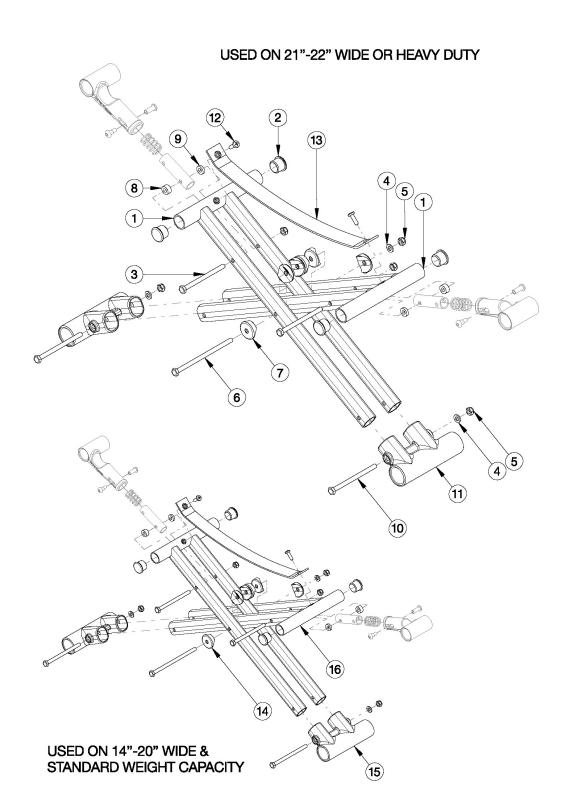
Oval-style cross braces effective 6/15/16 on 21" - 22" wide chairs and chairs with Heavy Duty option. Starting with serial numbers C4018744, C4HD002701. Round-style cross braces are used on 14" - 20" wide chairs with the Standard Weight Capacity. When changing from round-style to oval-style cross braces, lower frame pivots and cross brace hardware are required. Order kit 502177.
