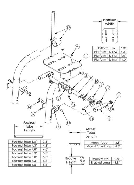
Use extended assemblies when chair has 2" or more Sling Position or 70°, 75° or 80° Front Frame Bend. Sizes based on straight frame/no taper. Not available with Heavy Duty Option
