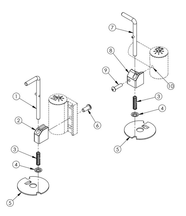
This design effective on serial numbers prior to TS010961, TSLW003890, TSHD003974, TSTR004740 and RG0018469 If replacing caster housings or caster lock mounting blocks with this Caster Pin Lock design, you must order new caster housings, caster lock mounting blocks and M5 split lock washers. See current Tsunami Caster Pin Locks page. Item Numbers 1, 2 and 6 are used on Catalyst models.
