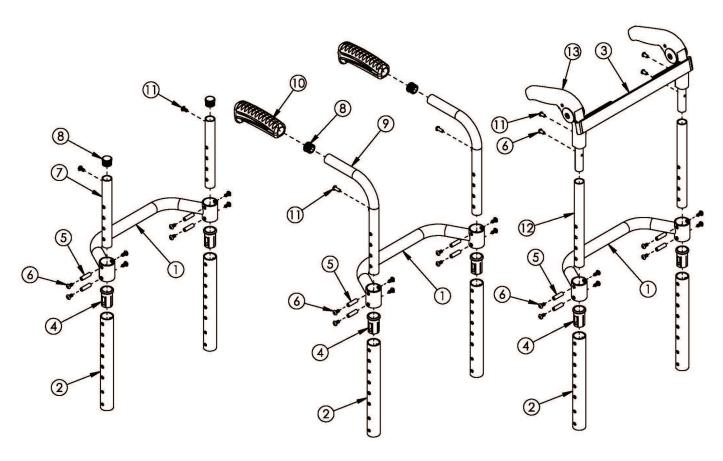
If chair was ordered with Rigid Locking Fold Down Back, please see Rigid Height Adjustable Back Post with Adjustable Height Rigidizer Bar page. Effective on Rogue starting with serial number RG0016612. If retrofitting to this backrest on Rogue, a new backrest mount and hardware may be required. Tension Straps (#3) are based on seat width and used in combination with back upholstery.
