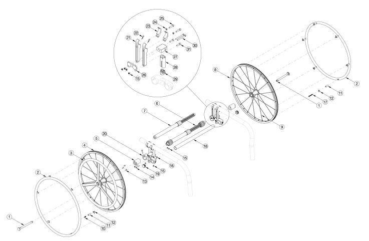
If retrofitting to add the One Arm Drive, new rear towers are required in addition to the complete One Arm Drive system and camber tube kit. Effective 5/13/2022, all One Arm Drives will be shipped with a close mounted handrim on the non-drive wheel. Most One Arm Drive kits do not include rear tires. Tires need to be quoted separately. Used on Rogue XP chairs invoiced starting on 3/12/25
