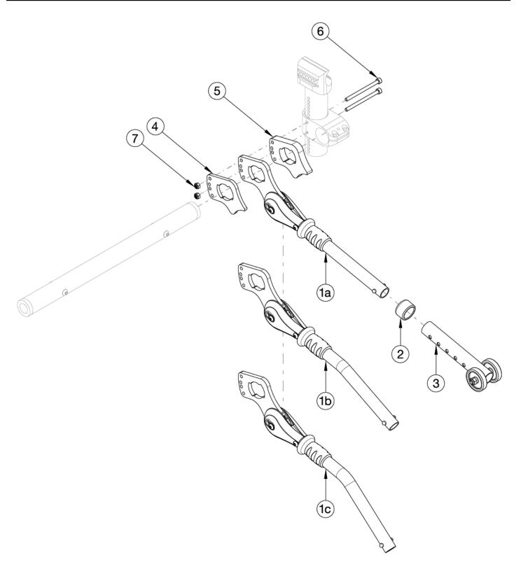
Contact Customer Service for chairs with more than 2" of variance between Front and Rear Seat Height. Complete assemblies contain "one" complete user activated anti-tip. Quantity two is required for a pair. A pair of User Activated Anti-Tips is not available if a tipping lever is present. Not available with One Arm Drive.
