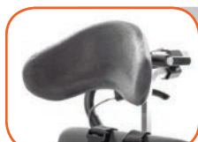
PY5626 Head Support-5"Hx8"W PY5628 Head Support-6"Hx10"W Cushion size is 5"Hx8"W (13x20cm), 6"Hx10"W (15x25cm). Depth range is +1" to -2.75" (+2 to -7cm) from backrest. Maximum height from seat is 24" (61cm).
