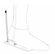
B. Drill holes using #17 or #16 drill bit. (nearest fractional size is 11/64")
